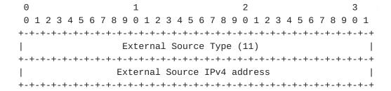
The new type of END-POINTS is External Source Node Type (11). The final value for the type will be assigned by IANA. This new type of END-POINTS object contains an external source node IPv4 address.
