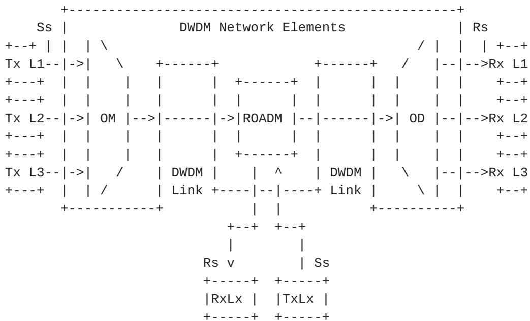
Ss = Sender reference point at the DWDM network element tributary output
