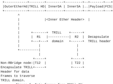
Figure 2 Data frames from TRILL-EN
