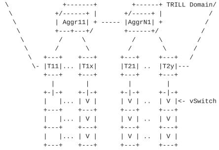
Figure 1 TRILL domain in typical Data Center Network
