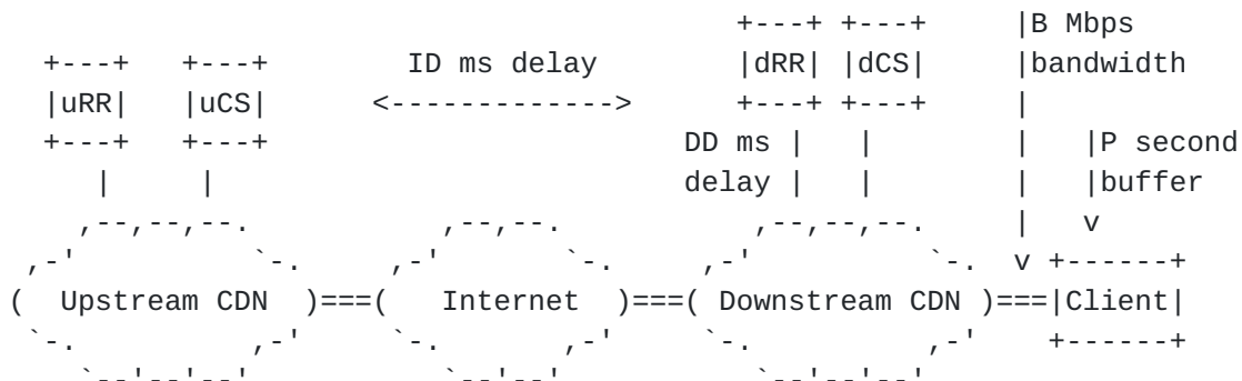
Figure 1: Evaluation scenario and parameters
