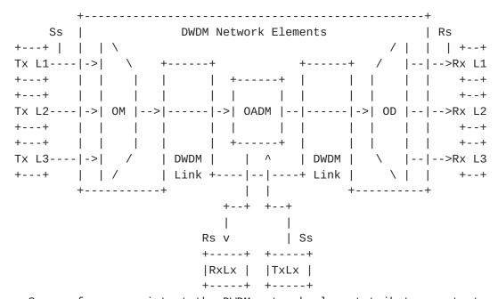
Ss = reference point at the DWDM network element tributary output Rs = reference point at the DWDM network element tributary input
