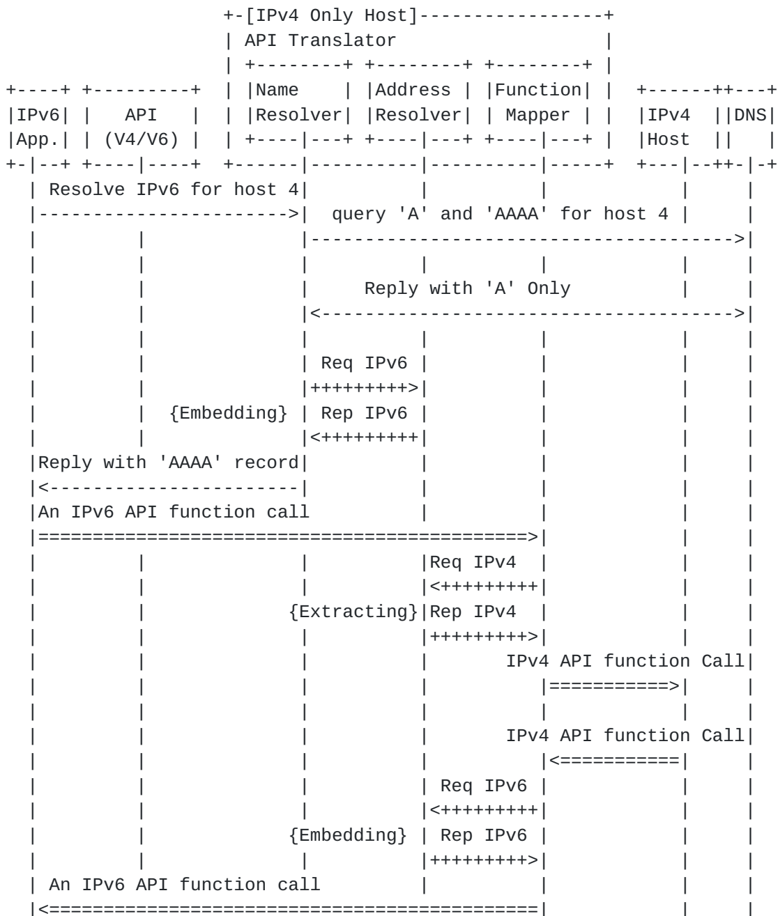
Figure 7: The behavior of the originator communicates with IPv4 Application
