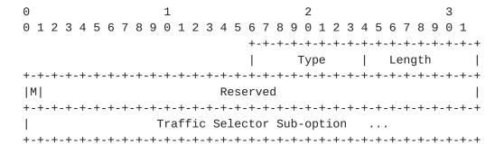
Figure 3: IPv4 Traffic Offload Selector Option
