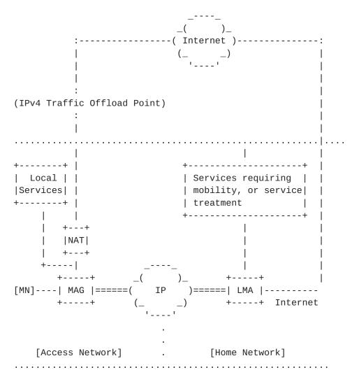
Figure 1: IPv4 Traffic Offload Support at the MAG
