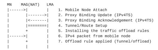
Figure 2: Exchange of IPv4 Traffic Offload Selectors
