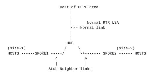
Simplified HUB Local RTR LSA contains only p2p link and a stub link with default or configured range
