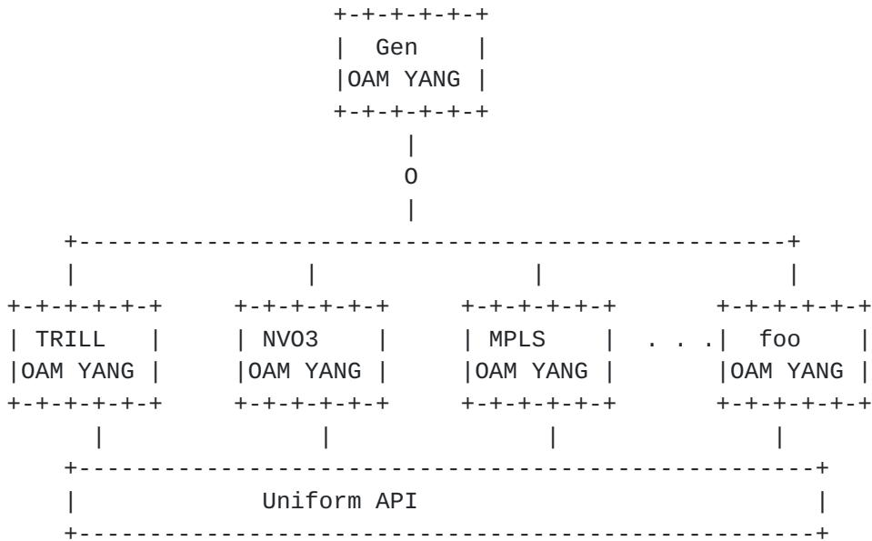
Figure 1 Relationship of TRILL OAM YANG model to Generic OAM YANG model
