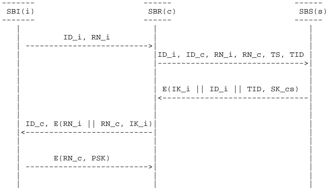
Figure 1 Message Exchange for PSK Reconfiguration
