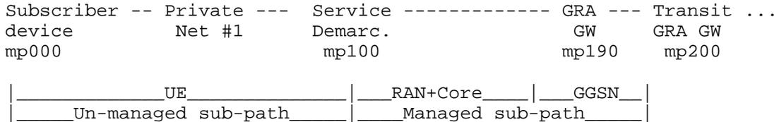
GRA = Globally Routable Address, GW = Gateway, UE = User Equipment, RAN = Radio Access Network, GGSN = Gateway GPRS Support Node.
