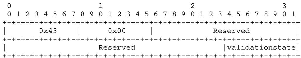
The value of the high-order octet of the extended Type Field is 0x43, which indicates it is non-transitive. The value of the low-order octet of the extended type field as assigned by IANA is 0x00. The Reserved field MUST be set to 0 and ignored upon the receipt of this community. The last octet of the extended community is an unsigned integer that gives the route's validation state [RFC6811]. It can assume the following values:
