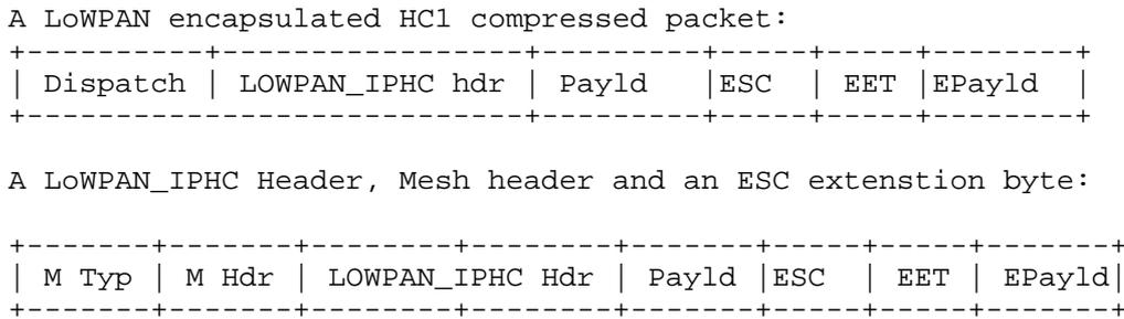
Figure 2: A 6lowpan packet with ESC Bytes
