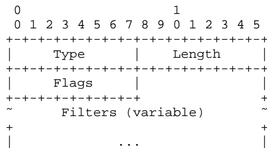
Figure 3: IS-IS FlowSpec Filters sub-TLV
