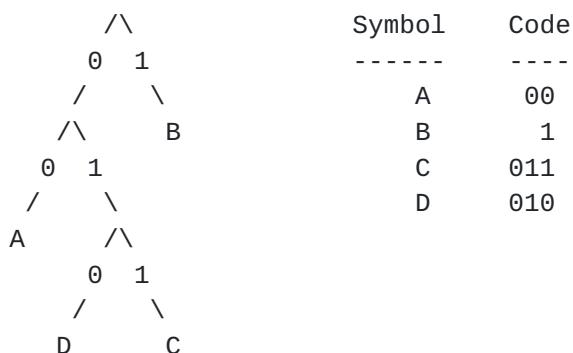
A parser can decode the next symbol from an encoded input stream by walking down the tree from the root, at each step choosing the edge corresponding to the next input bit.
