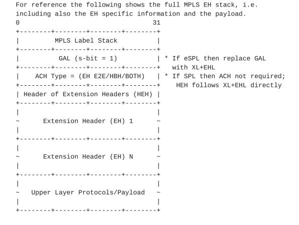
Figure 3: MPLS Extension Header (EH) Stack
