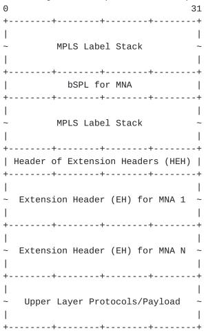
Figure 3: Label Stack with MNA
