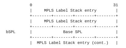
Figure 1: Example of Label Stack
