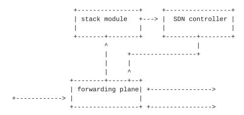
The forwarding plane is the datapath of the FSD. Before it working ,its forwarding table will be configurated by the SDN controller with NATCONF or OFPCONFIG protocol.
