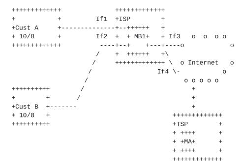
The main difference between the previous example and this one is that the physical MB, is subdivided into several logical MBs. Each logical MB has it's own interfaces and MB function profiles.
