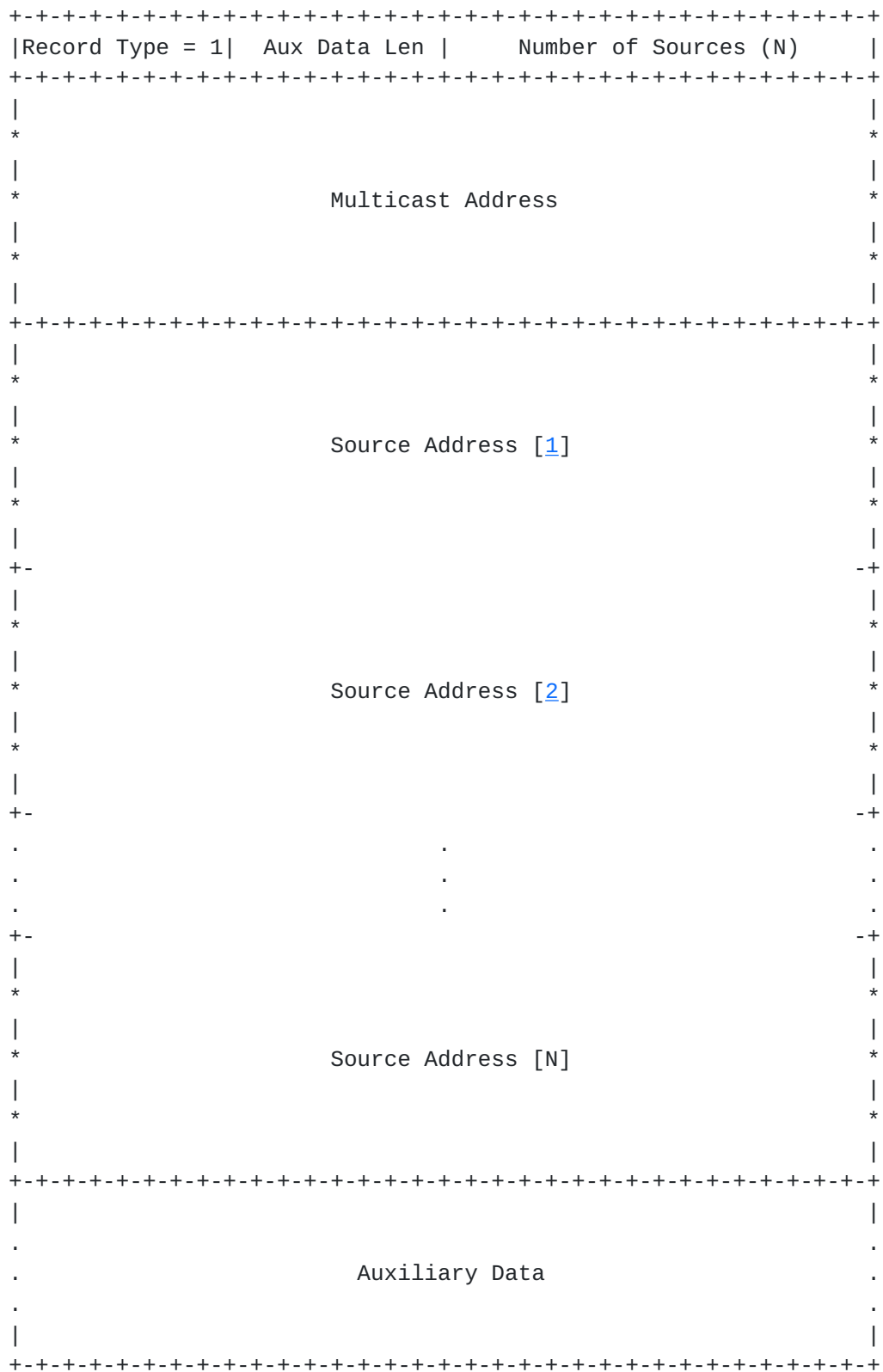
Figure 10: Multicast Address Record format
