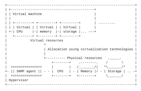
A hypervisor allocates virtual resources such as virtual CPUs, virtual memory, virtual storage devices, and virtual network interfaces to virtual machines from physical resources.
