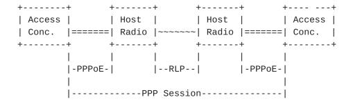
The capabilities of the RF links between RLP neighbors may vary over time due to mobility and environmental conditions. In many instances, the radio transmission system has limited buffering capability to handle capacity changes in the RLP sessions. To limit buffering in the radio transmission system, a session flow control mechanism is necessary to provide dynamic buffering feedback to the router.
