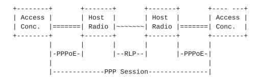
The capabilities of the RF links between RLP neighbors may vary over time due to mobility and environmental conditions. In many instances, the Host Radio has limited buffering capability to handle capacity changes in the RLP sessions. To limit buffering in the Host Radio, the PPPoE credit flow control mechanism provides dynamic buffering feedback to the access concentrator.
