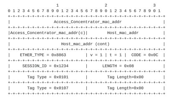
A PADQ packet with Metric Tag Type 0x0107:
