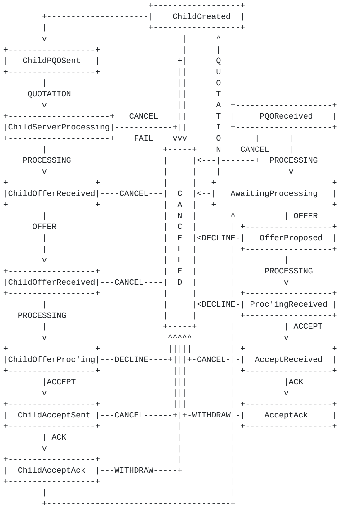
Figure 8: CPNP Finite State Machine (Server Side)
