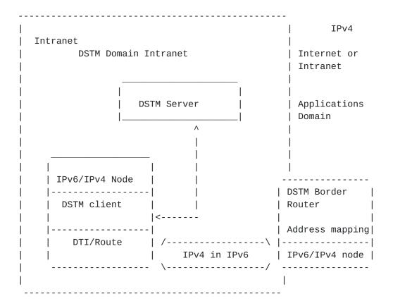
Figure 1: DSTM Architecture
