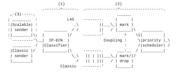
Figure 1: Components of an L4S Solution: 1) Isolation in separate network queues; 2) Packet Identification Protocol; and 3) Scalable Sending Host
