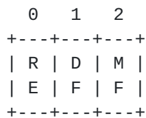
Figure 3: New Definition of the Re-ECN Extension (RE) Control Flag at the Start of Byte 7 of the IPv4 Header
