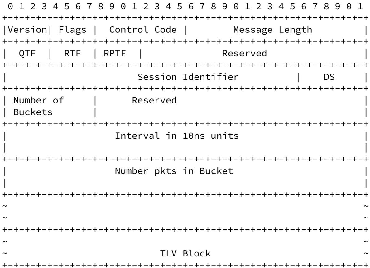
Figure 2: Bucket Jitter Measurement Message Format
