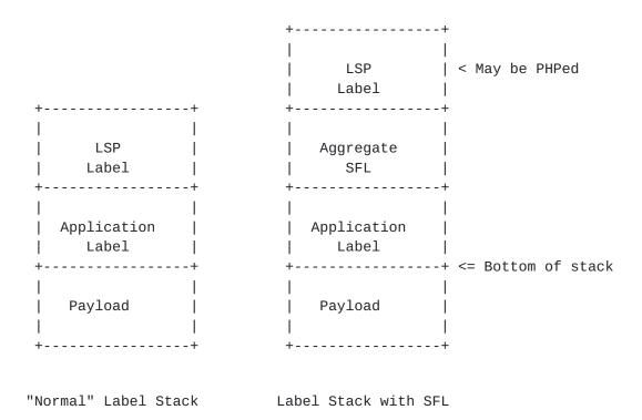
The Aggregate SFL is shown in the label stack depicted in Figure 3 as preceding the application label, however the choice of position before, or after, the application label will be application specific. In the case described in <a href="Section 3.1">Section 3.1</a>, by definition the SFL has the full application context. In this case the positioning will depend on whether the SFL action needs the full context of the application to perform its action and whether the complexity of the application
