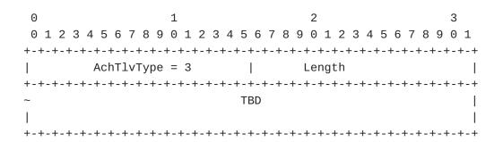
Figure 4: Label Switched Path Identifier
