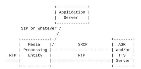
The "Media Processing Entity" is a network element that processes media. The "Application Server" is a network element that instructs the Media Processing Entity on what transformations to make to the media stream. The "ASR and/or TTS Server" is a network element that either generates a RTP stream based on text input (TTS) or returns speech recognition results in response to an RTP stream as input (ASR). The Media Processing Entity controls the ASR or TTS Server using SRCP as a control protocol.
