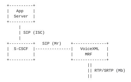
The above diagram is highly simplified and shows a subset of nodes typically involved in MRF interactions. It should be noted that while the MRF will primarily be used by the Application Server via the S-CSCF, it is also possible for calls to be routed directly to the MRF without the involvement of an Application Server.
