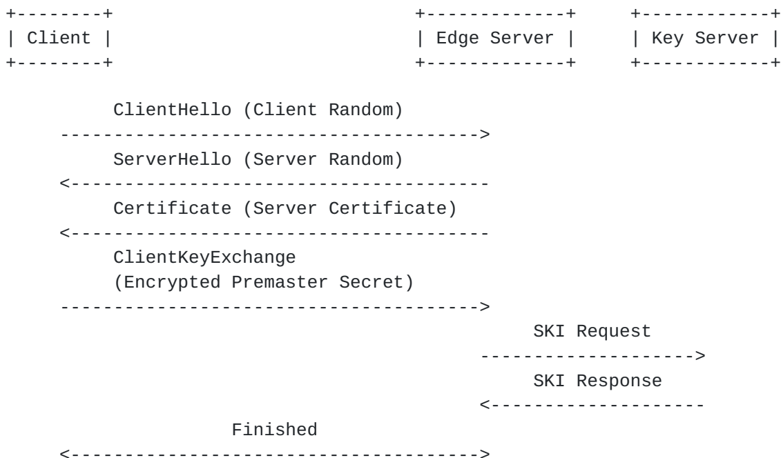
Figure 3: Message Flow for Static RSA Key Exchange
