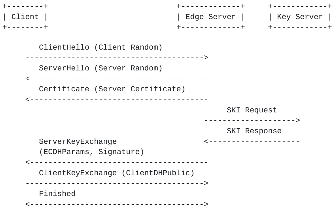
Figure 2: Message Flow for ECDHE Key Exchange
