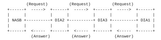
In this example, DIA3 traps messages generated from DIA2 towards DIA1, removes the AVPs added by DIA2 and inserts its own AVPs (possibly by trying to convince DIA1 to pay DIA3 for the services). This attack can be prevented by supporting a new Next-Hop AVP. In this case when NASB prepares a request it inserts a protected Next-Hop AVP which contains DIA2's identitity. DIA2 also adds a Next-Hop AVP with DIA1 as the next hop.
