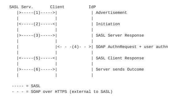
Figure 2: Authentication flow (no initial response)
