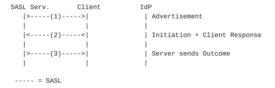
Figure 3: Authentication flow (with initial response)
