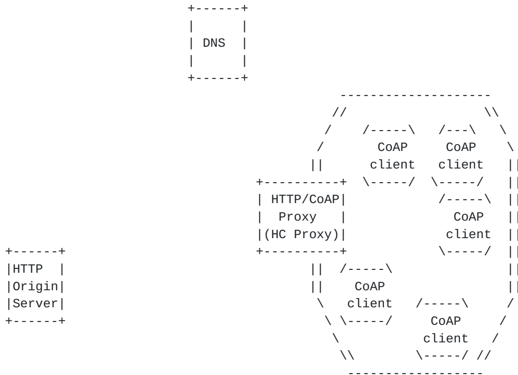
Figure 7: Client-side HC Proxy Deployment Scenario
