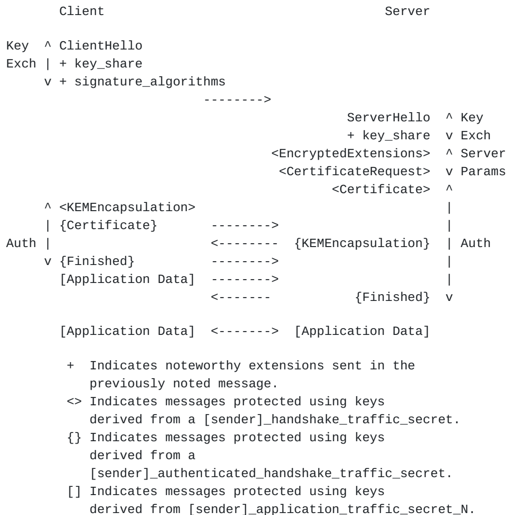
Figure 2: Message Flow for KEM-Authentication (KEM-Auth) Handshake with client authentication.
