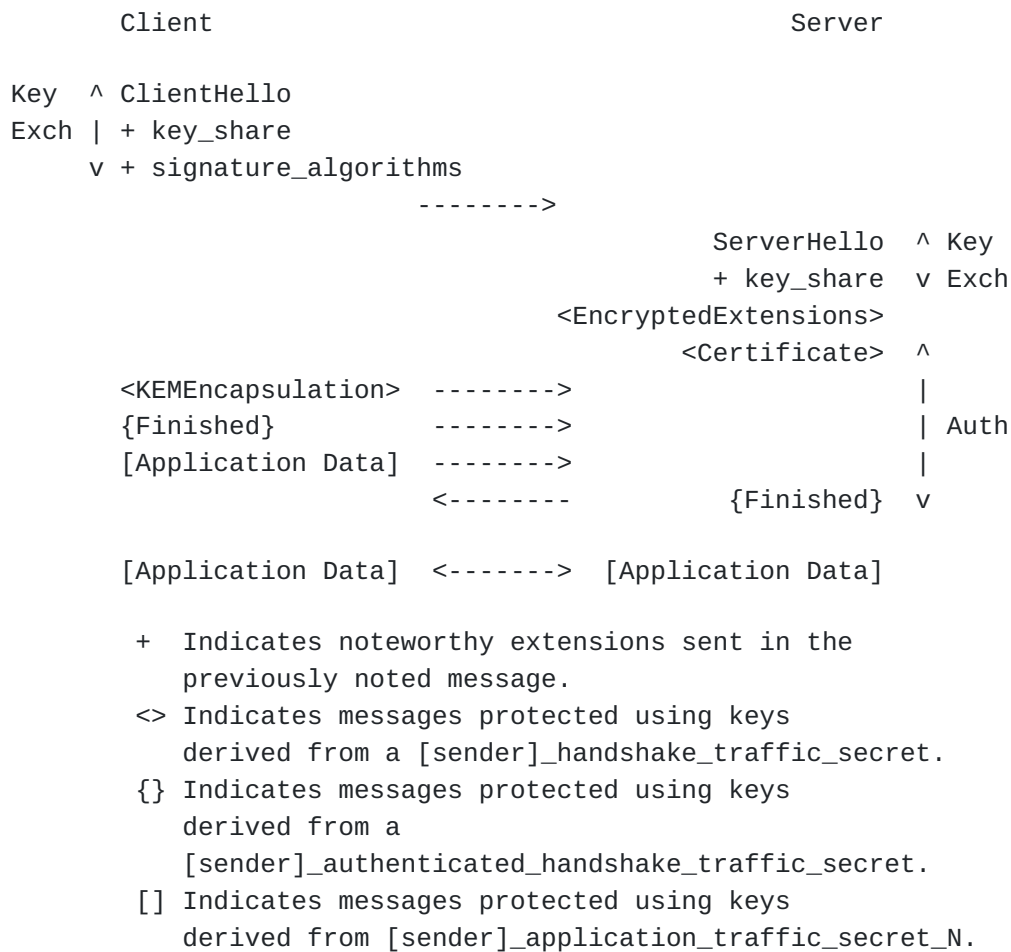
Figure 1: Message Flow for KEM-Authentication (KEM-Auth) Handshake without client authentication.
