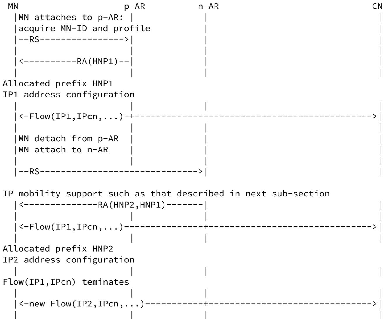
Figure 5. A flow uses the IP allocated from the network at which the MN is attached when the flow is initiated.
