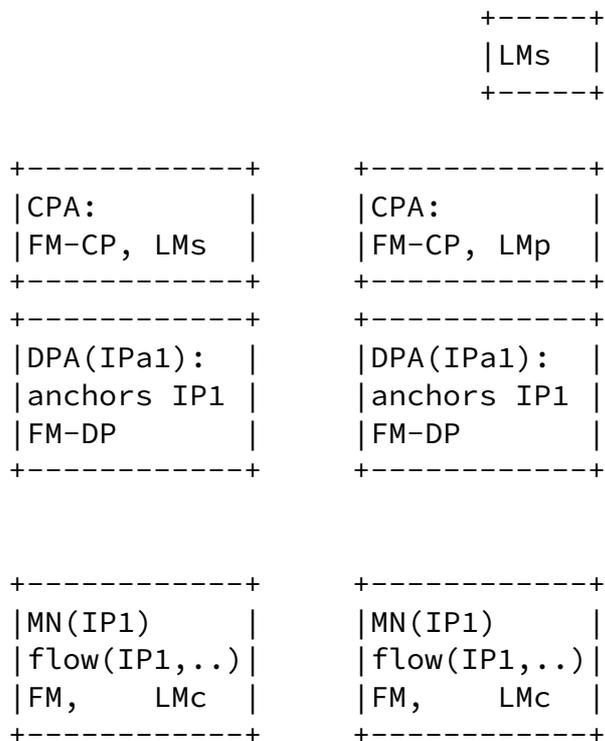
Figure 2. (a) FM-CP and LMs at CPA, FM-DP at DPA, FM and LMc at MN; (b) Separate LMs, FM-CP and LMp at CPA, FM-DP at DPA, FM and LMc at MN.
