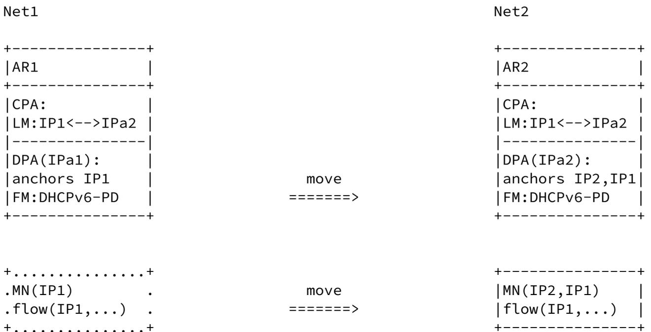
Figure 6. IP prefix/address anchor switching to the new network. MN with flow using IP1 in Net1 continues to run the flow using IP1 as it moves to Net2.
