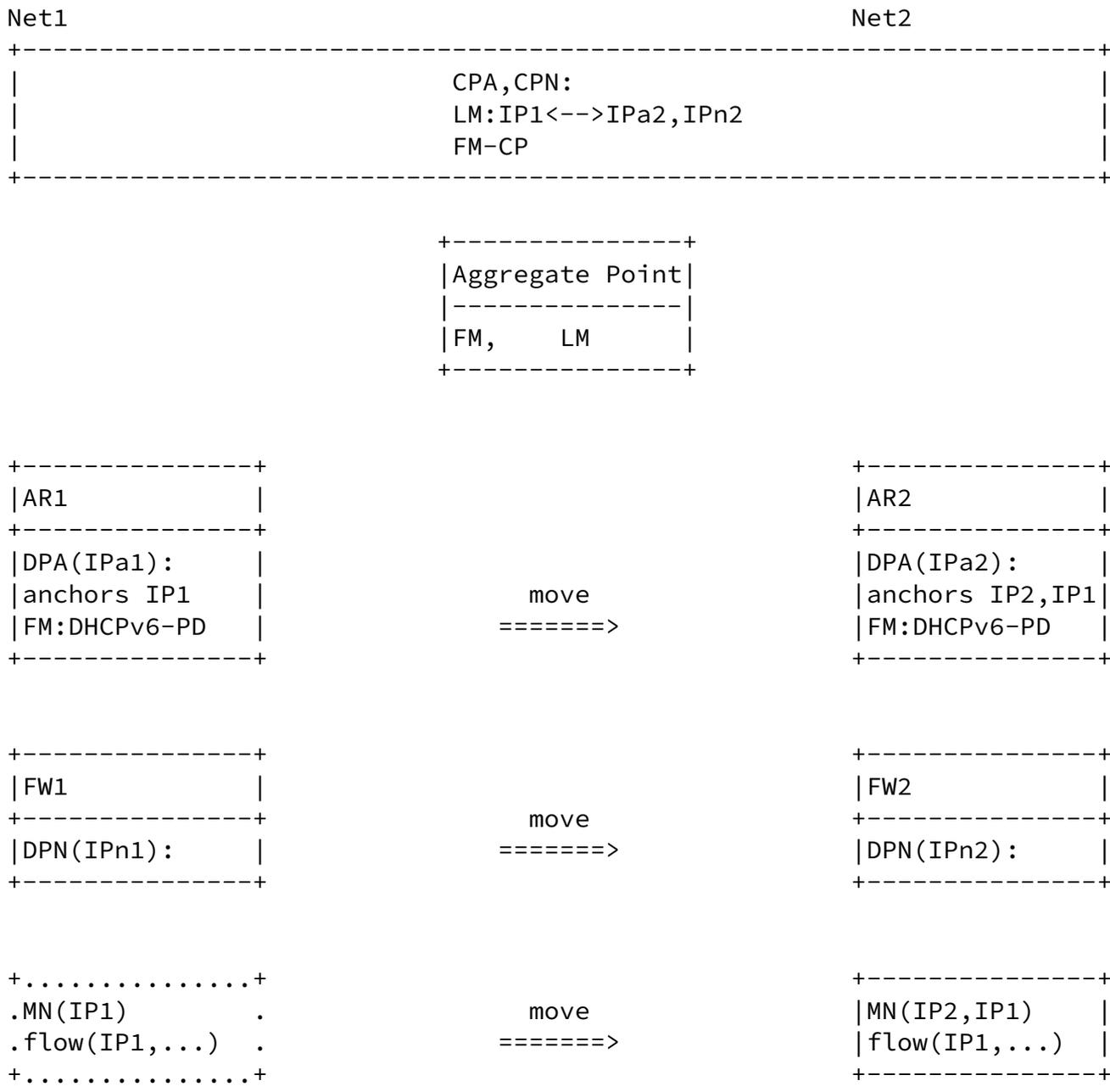
Figure 10. Mobility involving change of IP anchoring in a network with hierarchy in which the IP prefix allocated to the MN is anchored at an Edge Router supporting multiple access routers to which the MN may connect.
