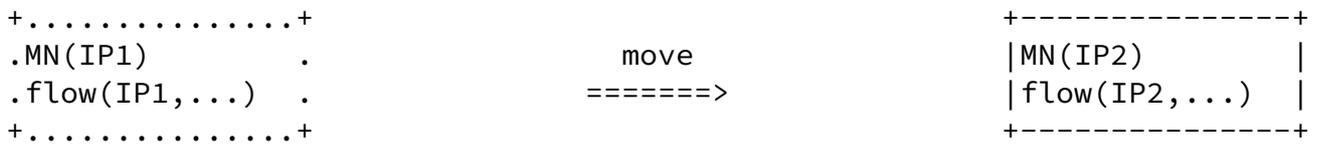
Figure 3. Changing to the new IP prefix/address. MN running a flow using IP1 in Net1 changes to running a flow using IP2 in Net2.
