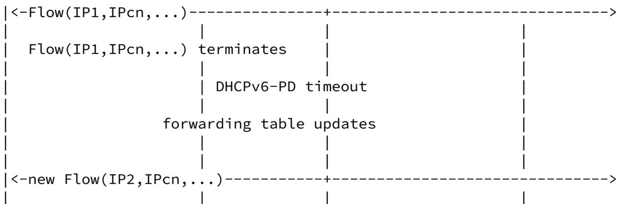
Figure 8. DMM solution. MN with flow using IP1 in Net1 continues to run the flow using IP1 as it moves to Net2.
