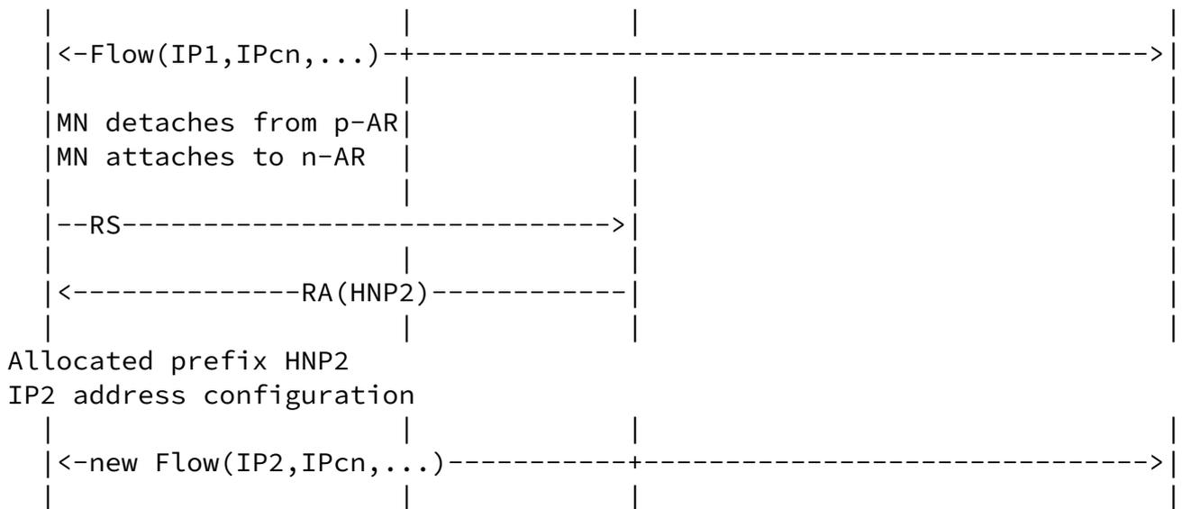
Figure 4. A flow uses the IP allocated from the network at which the MN is attached when the flow is initiated.
