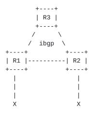
While R1 consistently selects the local static route as the best one, the route selection on R2 would be non-deterministic. As shown in the following figure, there are potentially two BGP paths A and B for X on R2, with Path A learned from R1 and Path B locally redistributed.
