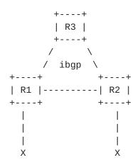
While R1 consistently selects the local static route as the best one, the route selection on R2 would be non-deterministic. As shown in the following figure, there are potentially two BGP paths A and B for X on R2, with Path A learned from R1 and Path B locally redistributed.
