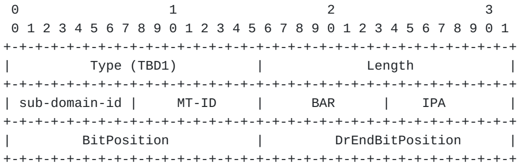
Figure 1: BIER-TE Sub-TLV in Router-Link TLV
