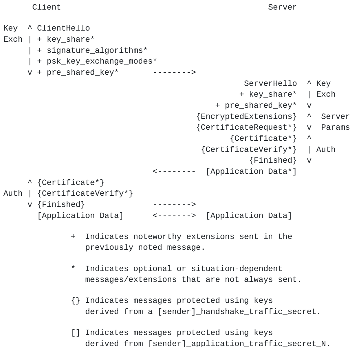
Figure 6: Message Flow for Full TLS1.3 Handshake
