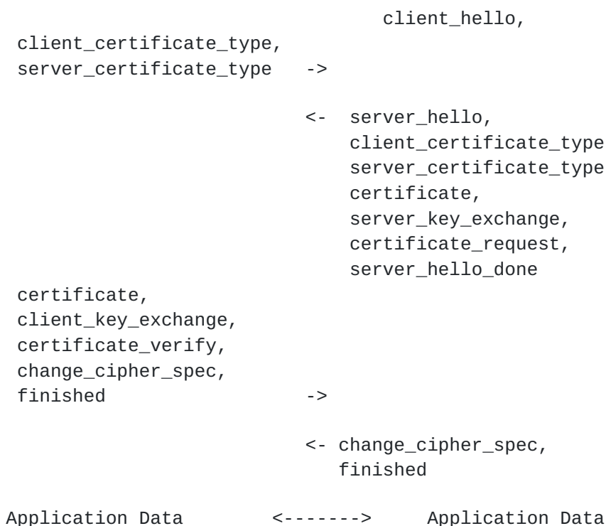
Figure 2: Basic Raw Public Key TLS Exchange
