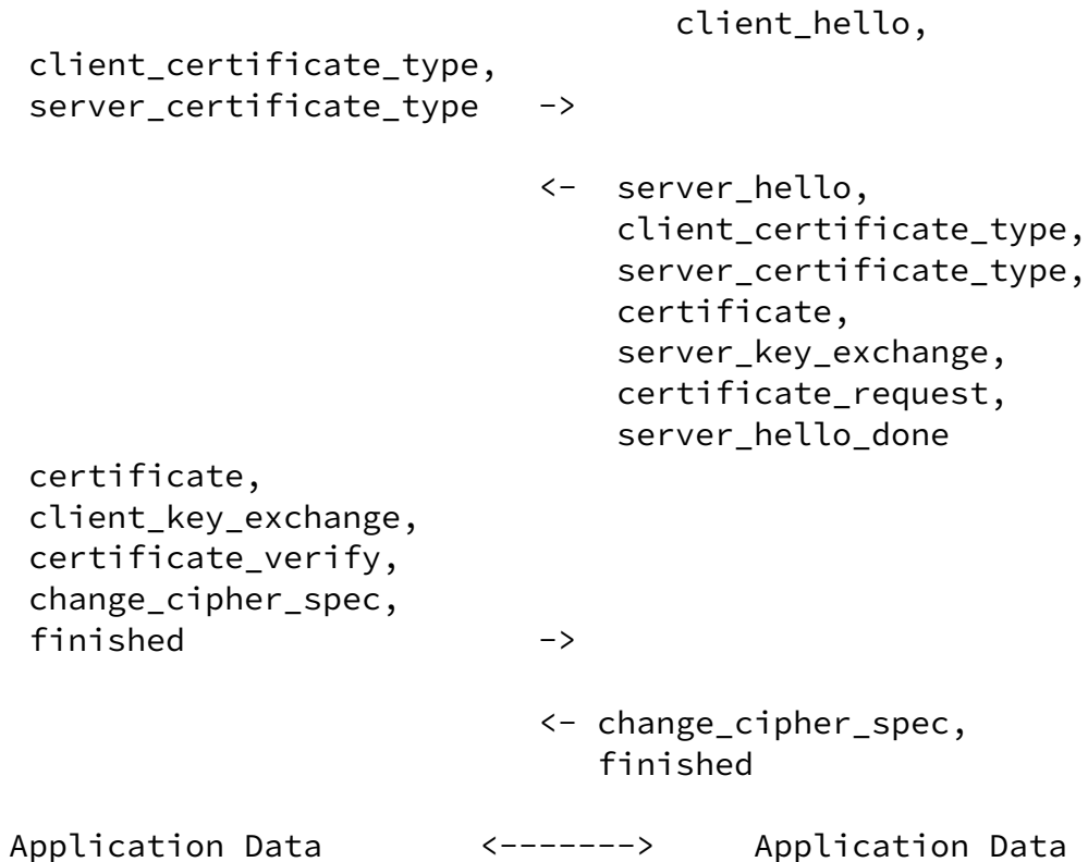
Figure 2: Basic Raw Public Key TLS Exchange
