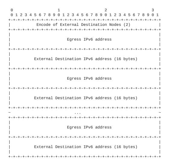
The object can only be carried in a PCReq message. A Path Request may carry at most one external destination nodes Object.
