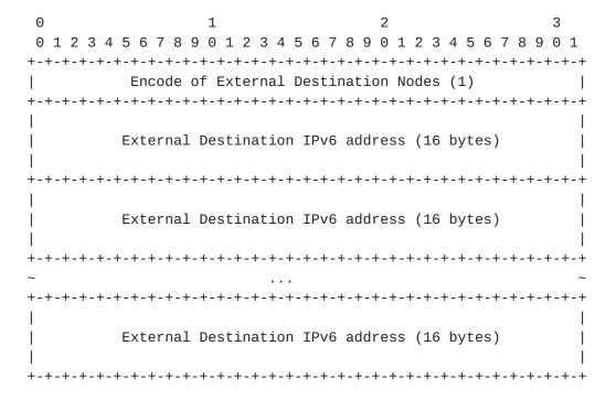
The format of the external destination nodes (EDN) object boby for IPv6 with the second type of encodes is illustrated below:
