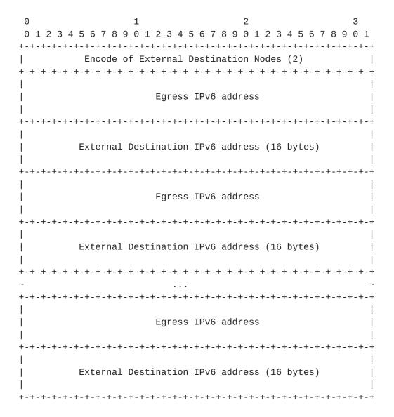
The object can only be carried in a PCReq message. A Path Request may carry at most one external destination nodes Object.
