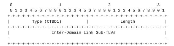
An Inter-Domain link TLV describes a single inter-domain link. It comprises a number of inter-domain link sub-TLVs for the information described in <a href="mailto:section4">section 4</a>, which are the sub-TLVs defined in <a href="mailto:RFC 3630">RFC 3630</a> or their equivalents except for the local IP address with mask length defined below.
