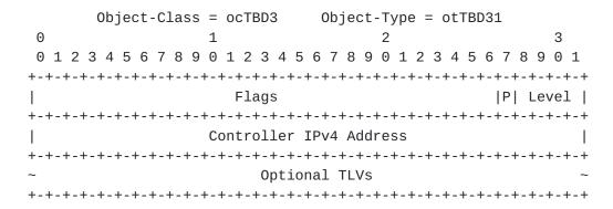
The RC-IPv4 object body has a 32-bit Flags field and a 32-bit Controller IPv4 Address. It may contain additional TLVs. No TLVs are currently defined.
