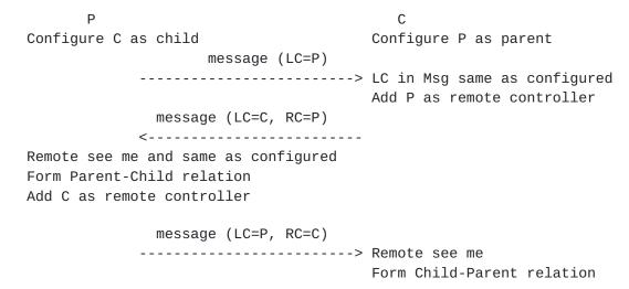
When C receives the message from P and determines that the local controller (LC=) P in the message is the same as the parent controller configured locally, it sends controller P a message containing local controller (LC=) C and remote controller (RC=) P.
