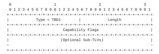
The type of the TLV is TBD1. It has a length of 4 octets plus the size of optional Sub-TLVs. The value of the TLV comprises a capability flags field of 32 bits, which are numbered from the most significant as bit zero. Each bit represents a capability.
