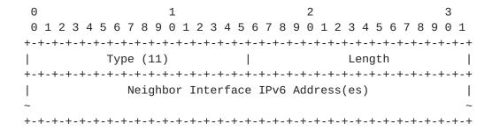
The Remote Interface IPv6 Address sub-TLV specifies the IPv6 address(es) of the neighbor's interface corresponding to the interdomain link. If there are multiple neighbor addresses on the link, they are all listed in this sub-TLV.
