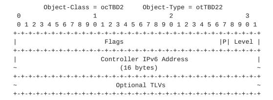
The LC-IPv6 object body has a 32-bit Flags field and a 128-bit Controller IPv6 Address. It may contain additional TLVs. No TLVs are currently defined.
