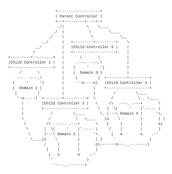
The parent controller communicates with these four child controllers and controls them, each of which controls (or is responsible for) a domain. Child controller 1 controls domain 1, Child controller 2 controls domain 2, Child controller 3 controls domain 3, and Child controller 4 controls domain 4.
